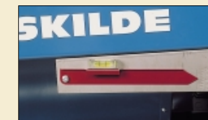
On one side of the machine is a spirit level to indicate the correct inclination. The inclination determines the flow velocity and thickness of the grain layer on the screens - and furthermore the cleaning efficiency.
