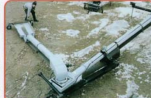
10" dia. swing arm conveyor. PTO driven.
