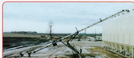
14" dia. x 85' track mounted conveyor fed with high capacity, 24" x 20' long straight undercar conveyor. Both are electrically driven.
