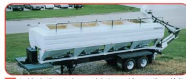
Electric over hydraulic controls give the operator remote load out control of each compartment.
