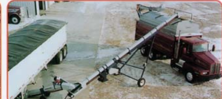
10" dia. x 35' long conveyor with 10" gooseneck style undercar conveyor. Both are gas driven.
