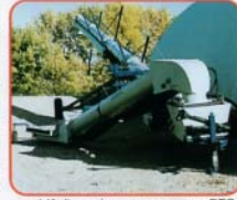
14" dia. swing arm conveyor. PTO driven.
