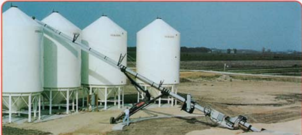
14" dia. x 75' pivot mount conveyor with available hydraulic wheel drive kit. Main conveyor is fed with a 14" dia. gooseneck style, pit model, undercar conveyor. The pit model conveyor has an 8' long receiving hopper.
